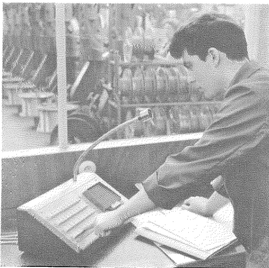
Figure 9—Master station of Dirigent 2/80 industrial intercommunication system.
