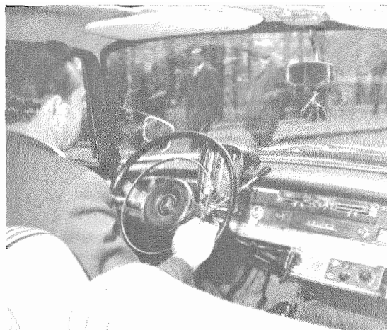
Figure 11—"Standafon" very-high-frequency radiotelephone equipment installed beneath the dashboard of an automobile.
